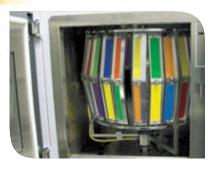
**Two Rotating Sample Rack Options** -The optional 2-tier rack system allows up to 60 total specimens to be exposed. The unique inclined shape of the rack maximizes irradiance and temperature uniformity across the entire sample surface area. The 2-tier rack can also be installed in any existing Ci3000+ instrument.
