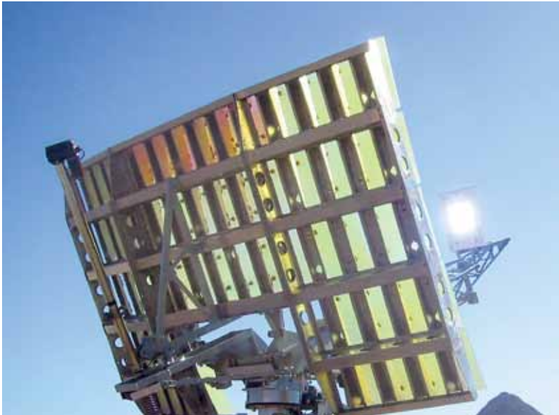
Figure 15 - Ultra-Accelerated Weathering System in Arizona
