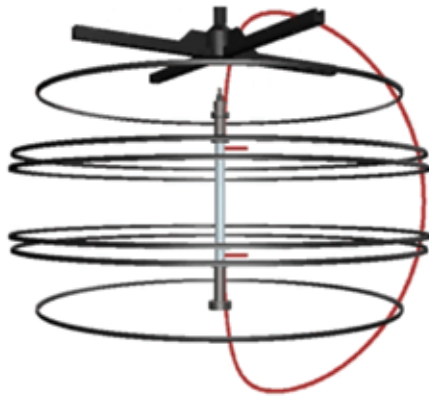
Figure 25 - Tiered specimen rack line of equal irradiance in relation to lamp
