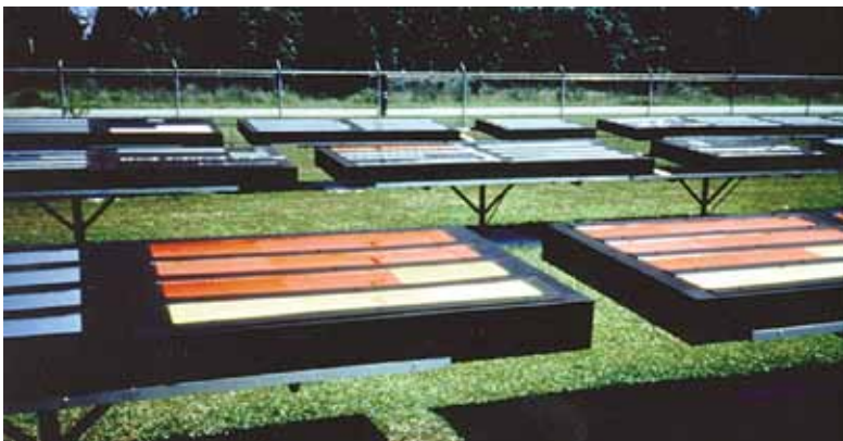
Figure 10 - "Black Box" exposure for automotive coatings
