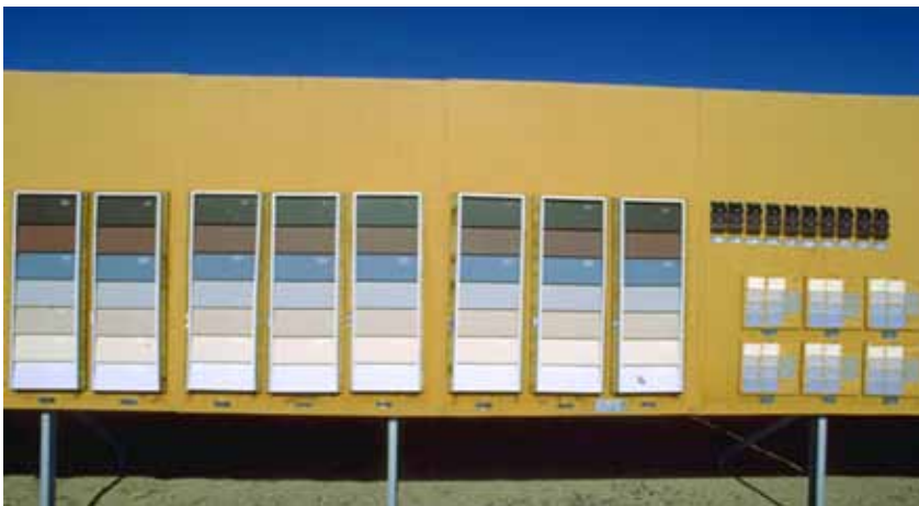
Figure 8 - Test specimens on a 90° vertical exposure rack
