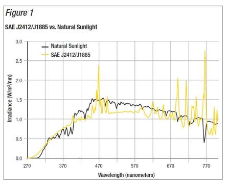
method is the ultimate criteria for UV performance and will override the results of the accelerated xenon testing per SAE J2412/ J1885.
