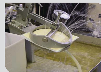
Water Leakage in the Hydrostatic Tester
