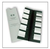
**Figure 3.** The AATCC and ISO Gray Scale for Staining. Ratings run from 1 to 5 in 0.5 unit steps.
