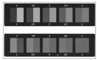
**Figure 2.** ISO/ASTM Gray scale for visual assessment of color change. Units range from 1 to 5 in 0.5 unit steps.
