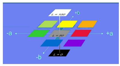
**Figure 4.** CIE L\*a\*b\* value defines a color by its 3-dimensional coordinates on this scale.
