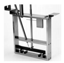
Easily interchangeable universal specimen holder for HDT testing in the Atlas HDV3
