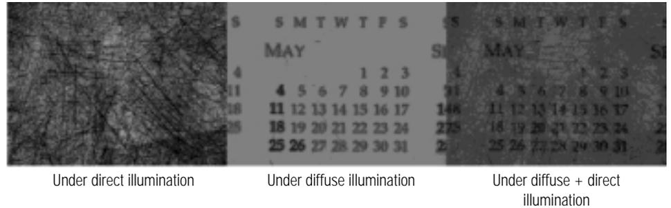
Figure 3: Selective viewing of surface structure using VIEEW direct/diffuse illumination
