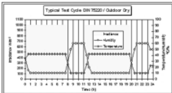
With the use of **KHS technology**, testing of automotive and other component parts and complete vehicles and assemblies can be accomplished in a short time frame, typically 18 to 30 days. A common test specification for performing component and full size automotive tests is DIN-75-220, titled “Aging of Automotive Components in Solar Simulation Units.”
