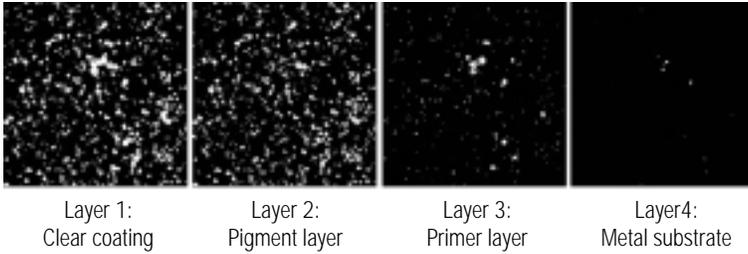
Figure 7: Chipping damage — each layer revealed
