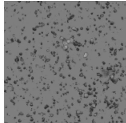
*Figure 6: Chipping damage in a multi-layer coating system — captured with VIEEW*
