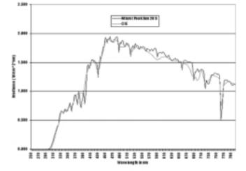
Figure 1: CIE vs. Atlas Peak Optimum Sunlight
