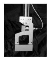
Instrumented Charpy Pendulum
