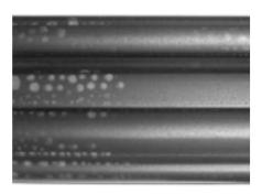
Photo of coated rubber sample after weathering testing in an Atlas Weather-Ometer<sup>®</sup>. White spots on the sample indicate that the test failed.
