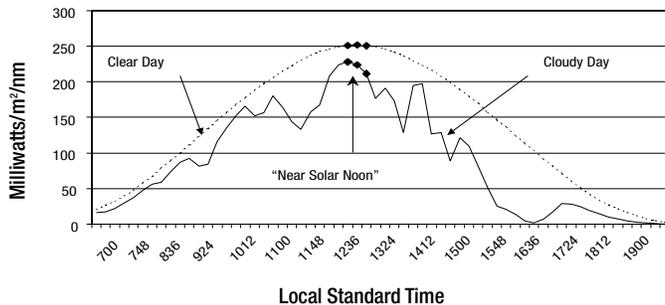
Figure 2. Solar noon intensities at 315.6 nm on a clear and cloudy day.
