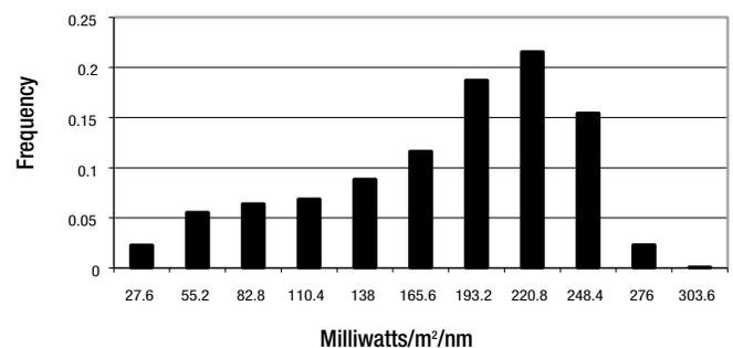
Figure 6. Histogram frequency distribution of solar intensities at 315.6 nm for 3 years in Miami (n = approx. 2780).
