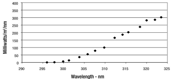
Figure 8. Proposed reference solar spectral power distribution for Miami, 45° south near solar noon.
