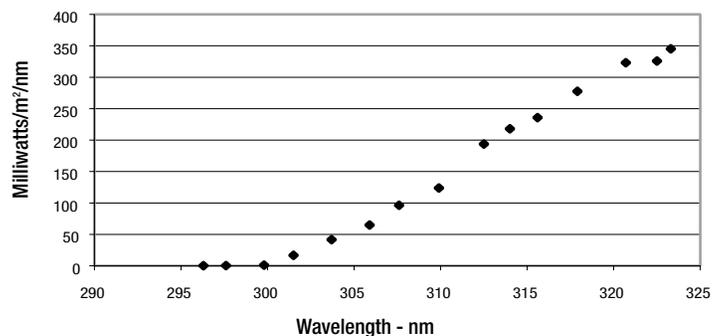
Figure 9. Proposed reference solar spectral power distribution for Phoenix, 45° south near solar noon.
