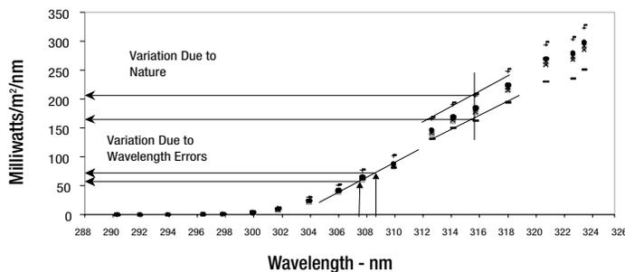
Figure 3. Effect of wavelength calibration errors on measured solar intensities.
