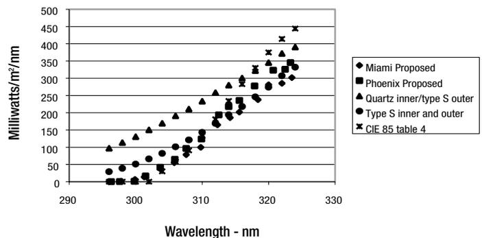
Figure 10. Comparison of the proposed reference SPDs to other light sources in weathering technology.
