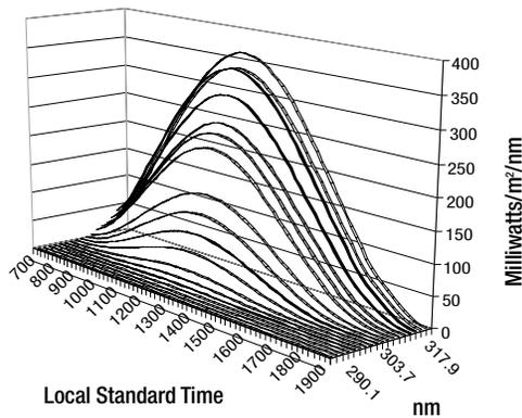
Figure 1. Example of daily solar spectral power distribution measurements made in June 1997 in Phoenix at 45° south.
