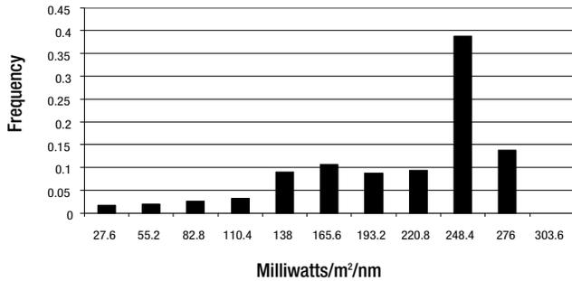
Figure 7. Histogram frequency distribution of solar intensities at 315.6 nm for 3 years in Phoenix (n = approx. 2970).
