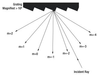
Figure 9: Multiple diffraction orders for a single wavelength
