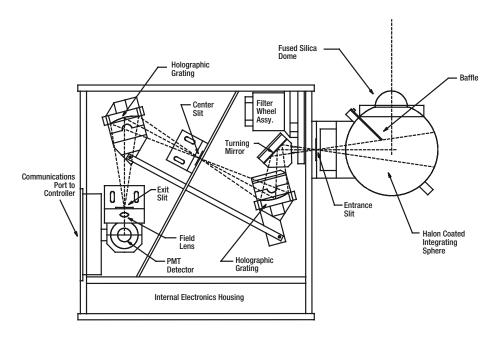
Figure 10: Double grating monochromator schematic
