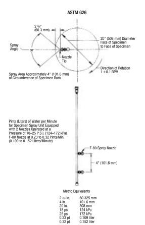
Specimen Spray Arrangement for Type A and AH Apparatus
