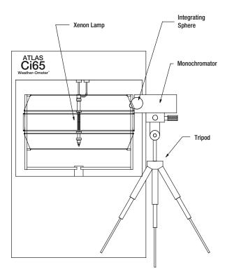
Figure 13: Spectroradiometric measurement in the Weather-Ometer<sup>®</sup> chamber
