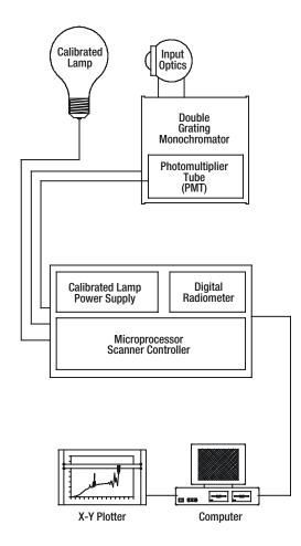
Figure 8: Spectroradiometer system block diagram
