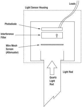
Figure 12: Light monitor sensor housing
