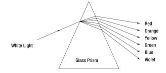
Figure 2: Dispersion of white light by a prism
