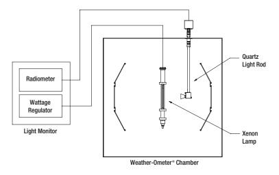
Figure 11: Controlled irradiance system
