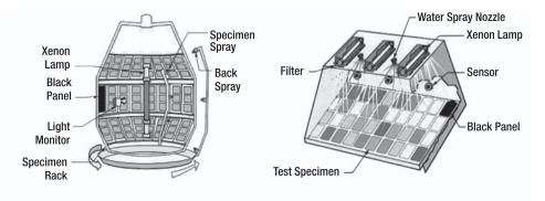
In calculating the cost of exposing specimens in a laboratory-accelerated environment, one should consider exposure uniformity and specimen throughput in the calculation. As stated, the Ci4000 has more than twice the exposure area of a Xe-3HS and due to the far superior uniformity in the Ci4000, the Xe-3HS will require more replicates than needed in the Ci4000.
