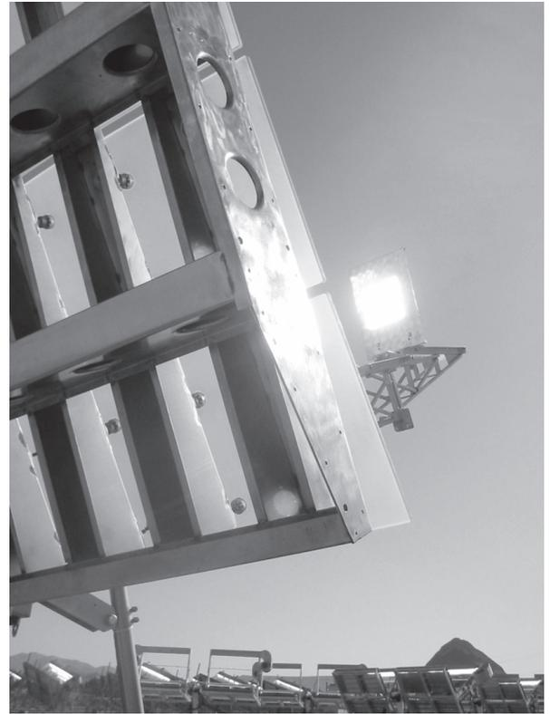
*Figure 5: Reflective facets, collector structure, and focused beam in target area*
