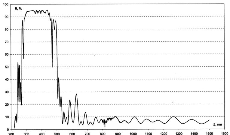
Figure 2: Reflectance spectrum of mirror facet
