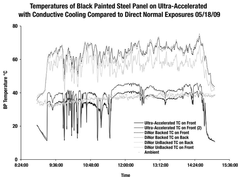
Figure 7: Ultra-accelerated and direct black panel temperatures
