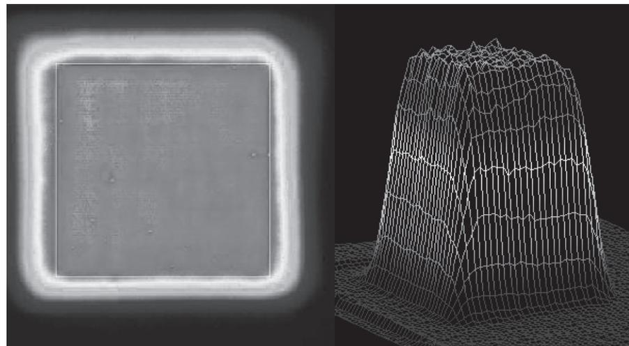
*Figure 6: Images from flux uniformity measurements*
