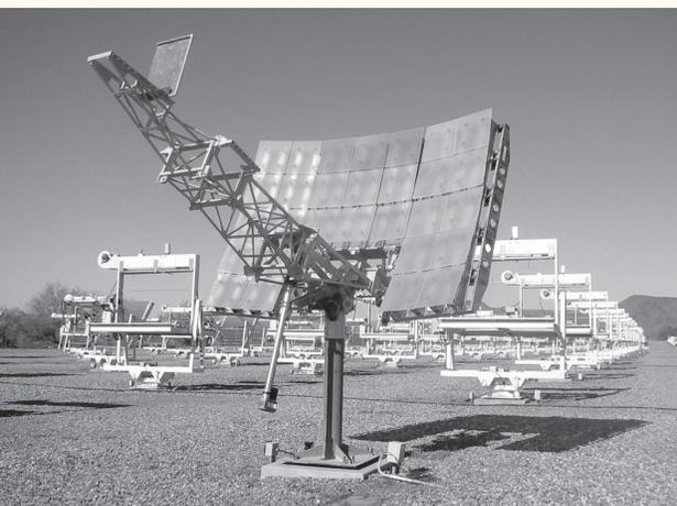
Figure 1: Ultra-Accelerated Weathering System (UAWS) installation, Arizona
