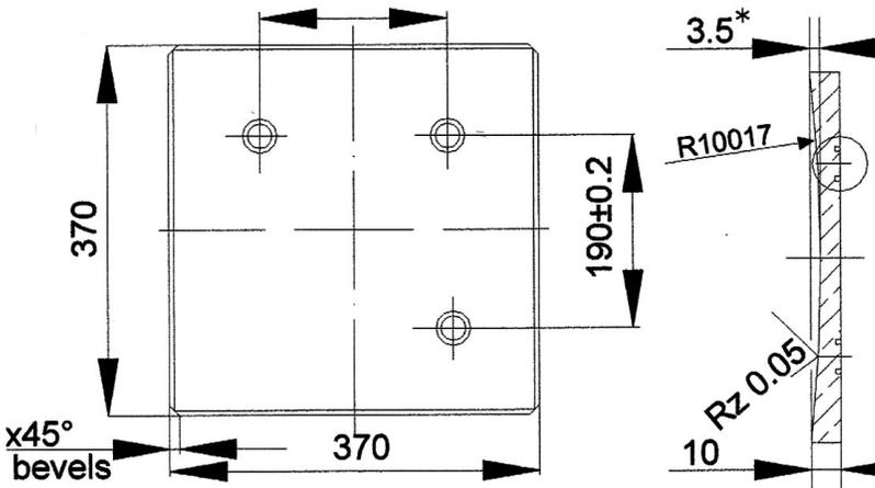
Figure 3: Reflective element construction (units in mm)
