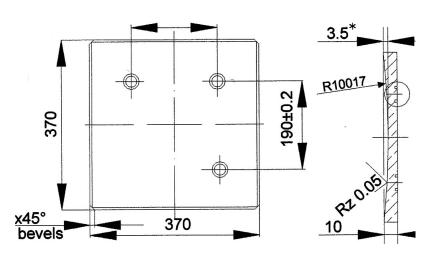
Figure 3: Reflective element construction (units in mm)
