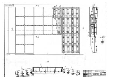
Figure 4: Collector support structure construction
