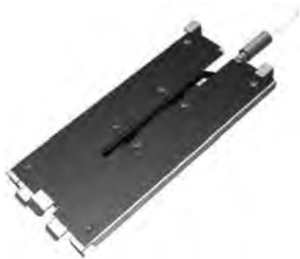
Figure 3 Graphical representation of an uninsulated black panel (BPT)
