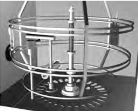
Figure 5 Components of the Specific Specimen Surface Temperature (S 3 T) system
