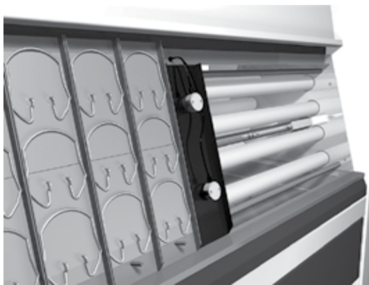
Figure 7: Inside of an Atlas UVTest showing UV lamps, Black Panel Temperature Control and ergonomically designed specimen retention clips
