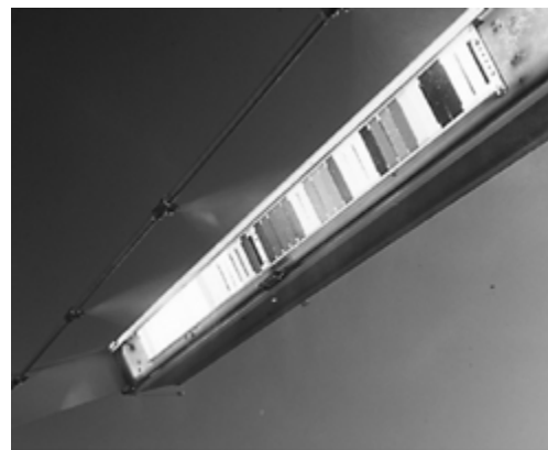
Figure 5: EMMAQUA® water sprays provide thermal shock or night time dew wetting
