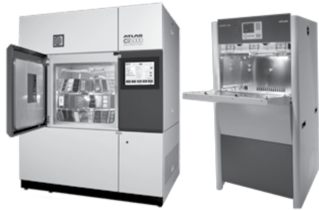
Figure 6: Ci5000 Weather-Ometer® rotating rack xenon instrument and SUNTEST® XXL+ flatbed xenon instrument
