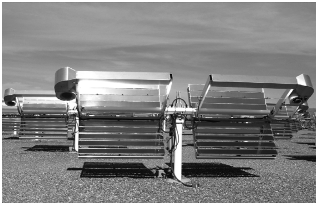
Figure 4: EMMAQUA® solar concentrator for accelerated weather testing
