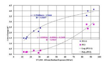
**Figure 6.** A fit of the data at three irradiances for two polyurethanes,  $\Delta E$  versus radiant exposure shows good reciprocity.
