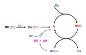
Figure 2. Photolysis is an initiating step in polymer autooxidative degradation, but subsequent reactions may be influenced by secondary factors independent of irradiance.
