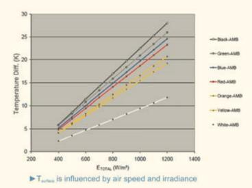
Figure 1. Excellent linearity of color coated panel surface temperature control achieved with increasing irradiance in Xenotest® Beta [4]
