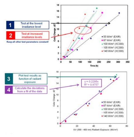
Figure 3. Simplified reciprocity validation method using ORWET [11] orange lacquer coating standard reference material; ISO 4892-2 xenon test method (no water spray). Note that the property change ( $\Delta E$ ) is very linear with radiant exposure for this material [12].
