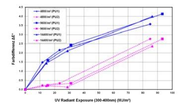
Figure 5. Although the property change is not linear with radiant exposure, the amount of the change at equal radiant exposures, but different irradiances, was similar; this is an indication that reciprocity was obeyed. A curve fit showed excellent R<sup>2</sup> values (R<sup>2</sup> is the square of the Pearson correlation coefficient, r).
