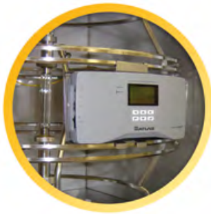
LS-200 spectroradiometer mounted on Ci chamber rack
