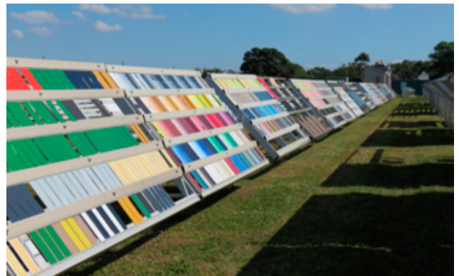
Figure 3: Samples on outdoor exposure racks at Atlas' South Florida Test Site
