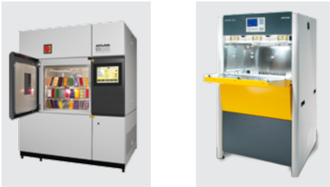
Figure 12: Ci5000 Weather-Ometer® (rotating rack) and SUNTEST XXL+ (flatbed) in Atlas' Accelerated Weathering Laboratory in Mount Prospect, IL
