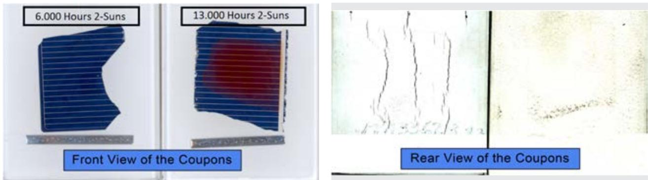
**Figure 8.** Picture of the front view and the rear view of 2 different coupons of “Glass/EVA/Piece of Cell + Ribbon/EVA/Backsheet” after 6,000 hours (left) and 13,000 hours (right) 2-Suns. The rear view of the coupons shows a backsheet of poor design which is cracking in the area of the piece of PV cell because of thermal aging degradation and thermal shock (rain cycles).
