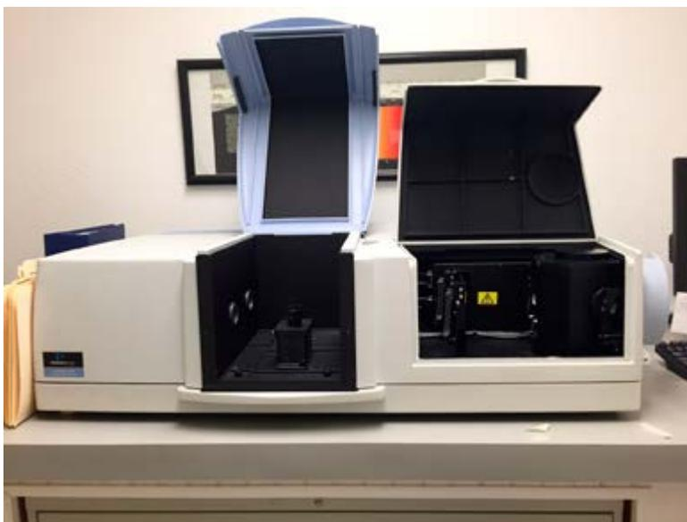
Figure 1: The Perkin Elmer Lambda 950 spectrophotometer is used to perform spectral transmittance, reflectance, and absorptance measurements.
