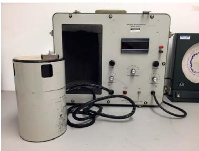
Figure 2: The Gier-Dunkle DB-100 is used to perform thermal emittance measurements.
