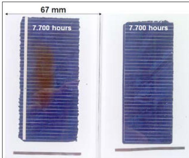
**Figure 4.** 7,700 hours 2-Suns weathering of 2 coupons of “Glass/EVA/Cell + Ribbon/Rear Encapsulant/PE-PA-PP Backsheet” with same EVA. Left: Development of a brown area between glass and cell at the center ( $O_2$  depletion); Right: No development of such a brown area.
