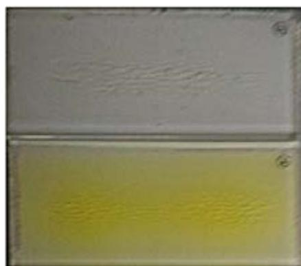
**Figure 3.** Discoloration in Damp Heat of a “Glass/EVA/PE-PA-PP Backsheet” coupon, where the backsheet comprises an efficient anti-oxidant with an isocyanurate ring structure. Top: EVA without TAIC; Bottom: EVA with TAIC.
