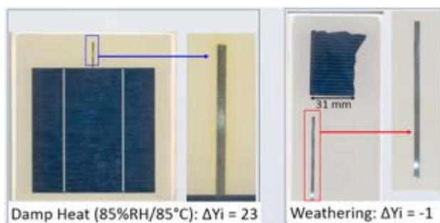
**Figure 1.** Left: 1,000 hours DHT (severe yellowing/discoloration, especially along ribbon); Right: 21,000 hours weathered coupon (no discoloration or corrosion of either fingers or ribbon)
