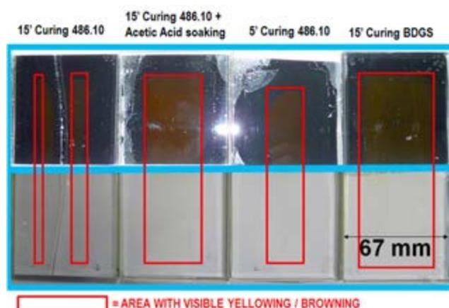
**Figure 7.** Picture of “Glass/EVA/Glass” samples after 7,000 hours 2-Suns weathering test. The bleaching distance depends on EVA formulation and its “degradation” state.
