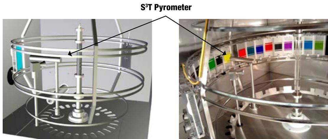
*Figure 1: Pyrometer in a weathering instrument used to measure the surface temperature of the exposed samples. The temperature is recorded while the samples rotate past the pyrometer.*
