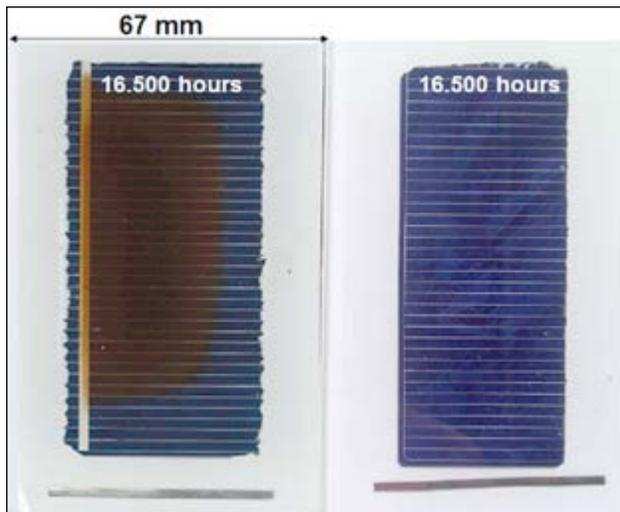
**Figure 5.** 16,500 hours 2-Suns Weathering of 2 coupons of “Glass/EVA/Cell + Ribbon/Rear Encapsulant/PE-PA-PP Backsheet” with same EVA. Left: Development of a brown area between glass and cell at the center ( $O_2$  depletion); Right: No development of such a brown area.
