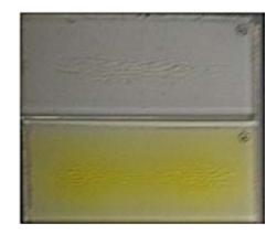
Figure 3. Discoloration in Damp Heat of a "Glass/EVA/PE-PA-PP Backsheet" coupon, where the backsheet comprises an efficient antioxidant with an isocyanurate ring structure. Top: EVA without TAIC; Bottom: EVA with TAIC.
