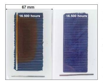
Figure 5. 16,500 hours 2-Suns Weathering of 2 coupons of "Glass/EVA/Cell + Ribbon/Rear Encapsulant/PE-PA-PP Backsheet" with same EVA. Left: Development of a brown area between glass and cell at the center (O<sub>2</sub> depletion); Right: No development of such a brown area.
