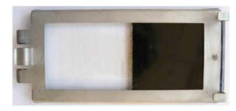
Figure 6. Picture of the coupon in its holder left part is "Glass/EVA/Glass" and right part is "Glass/EVA/Glass/EVA/Black Backsheet."
