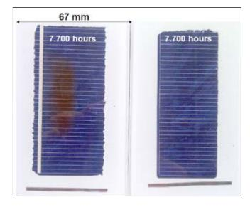
Figure 4. 7,700 hours 2-Suns weathering of 2 coupons of "Glass/EVA/Cell + Ribbon/Rear Encapsulant/PE-PA-PP Backsheet" with same EVA. Left: Development of a brown area between glass and cell at the center (O<sub>2</sub> depletion); Right: No development of such a brown area.
