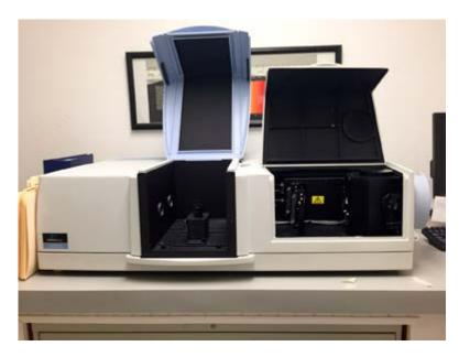
Figure 1: The Perkin Elmer Lambda 950 spectrophotometer is used to perform spectral transmittance, reflectance, and absorptance measurements.
