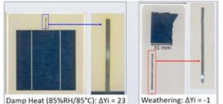
Figure 1. Left: 1,000 hours DHT (severe yellowing/ discoloration, especially along ribbon); Right: 21,000 hours weathered coupon (no discoloration or corrosion of either fingers or ribbon)
