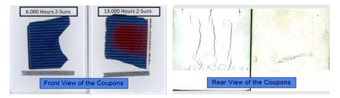
Figure 8. Picture of the front view and the rear view of 2 different coupons of "Glass/EVA/Piece of Cell + Ribbon/EVA/Backsheet" after 6,000 hours (left) and 13,000 hours (right) 2-Suns. The rear view of the coupons shows a backsheet of poor design which is cracking in the area of the piece of PV cell because of thermal aging degradation and thermal shock (rain cycles).
