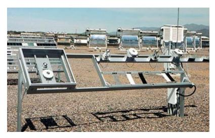
One of the radiometer racks at Atlas' DSET Laboratories, Arizona with various measuring instruments.
