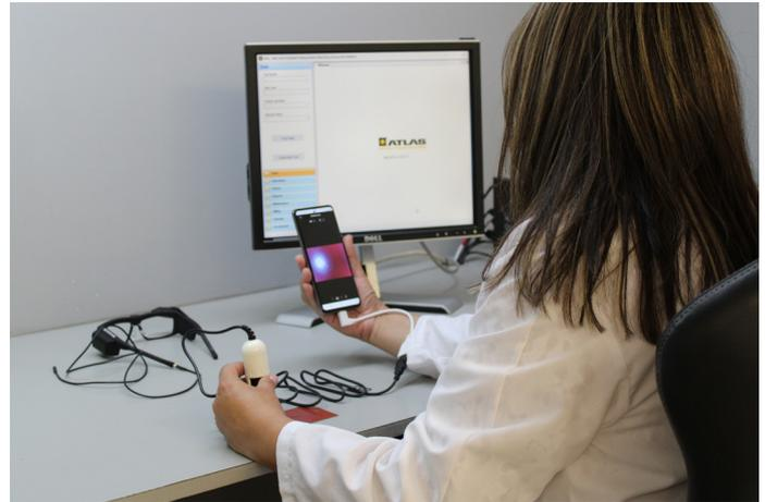
*The digital microscope (up to 60x) can be used to magnify specific degradation modes*
