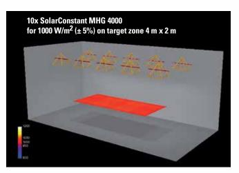
SolarConstant MHG 4000/2500 are often used for solar simulators integrated into climatic chambers. The tool of choice to determine thermal heating effects of solar radiation, such as fit and finish, dimensional stability or thermal transmission. Further to identify photodegradation effects of polymers and coatings such as change of color, gloss, haptics or physical strength. Further, testing PV module performance.
