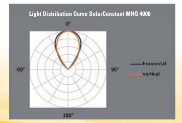
SolarConstant MHG 4000/2500 unit ideal for solar simulators of any size. Special reflectors guarantee high uniformity on the target area.
