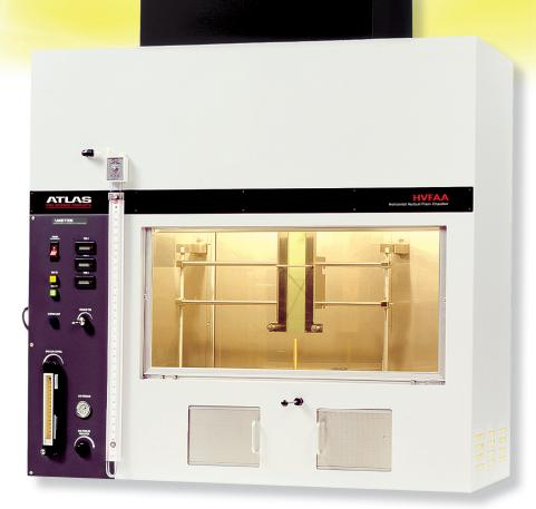
Atlas' HVFAA Horizontal Vertical Flame Chamber accurately determines the flammability of cabin compartment materials and electric wire. The chamber is designed to perform Bunsen burner tests in accordance with FAA's *Aircraft Material Fire Test Handbook, Revision 3,* DOT/FAA/TC-17/55, chapters A1, C1, D1, D2, and D8 (FAR 25.853, 25.855, 25.1359).
