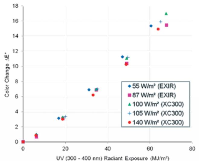
ORWET Orange coatings exposed in a Xenotest® Alpha at different irradiance levels according to ISO 4892-2 without rain cycle. Color difference as function of time and radiant exposure (XC300 = XENOCHROME® 300 daylight filter, EXIR = daylight extended infrared filter for better temperature control at low irradiance levels).
