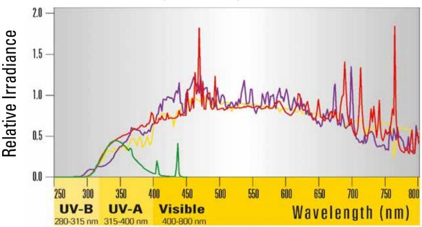
UVA-340 Fluorescent Lamp As used in the Atlas UVTest\* Metal Halide Global
