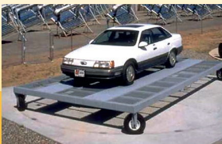
Sun-tracking carousel for automotive temperature measurement programs
